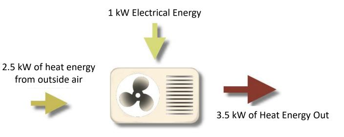
Heat Energy Out / Electrical Energy = COP 3.5kW / 1 kW = 3.5 COP
