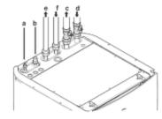
Piping Guidelines Minimum: 3m Maximum: 30m (ventilation required if 27m+) Height Difference: 20m Min Flow Rate: 12L/min
