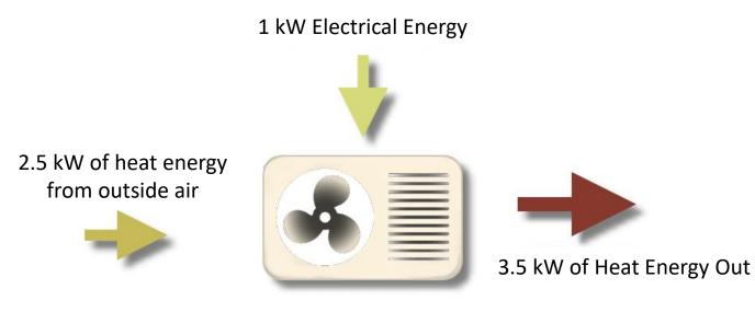
Heat Energy Out / Electrical Energy = COP 3.5kW / 1 kW = 3.5 COP **Or 350% Efficiency**
