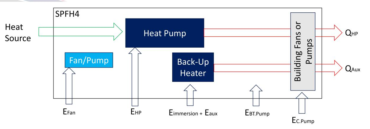
SPFH3 = QHP + QAux / EHP + EFan + Eimmersion + Eaux + EBT.Pump + EC.Pump
