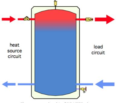
Flow rate to load is GREATER than flow rate from heat source. Cooler water moves upward in tank. Heat is being extracted from tank.
