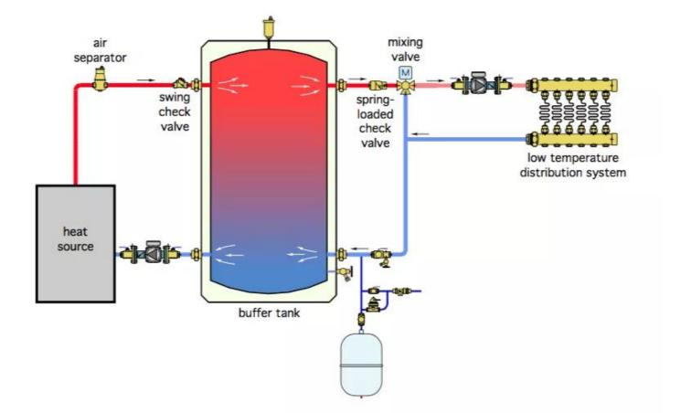
A Buffer Tank is designed to help reduce cycling of a heat pump or to reduce the compressor switching off/on (no more than 3 times per hour)
