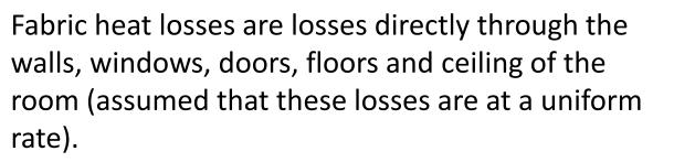
Fabric Heat Loss (Watts) = [Area (m<sup>2</sup>)] x ['U' Value (W/m<sup>2</sup>x°C)] x [ΔT (°C)]
